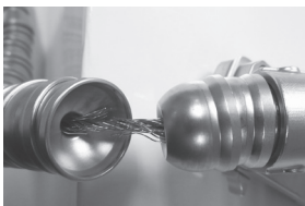
Figure 7 - Cable demonstrating fatigue and fraying
