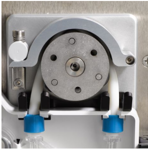
Figure 7-8: Tubing properly loaded onto a pump
