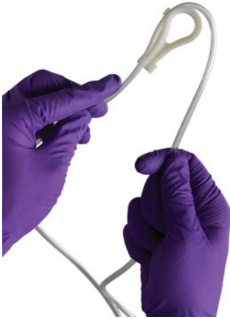
Figure 5-4: Removing the sample coil strain relief
