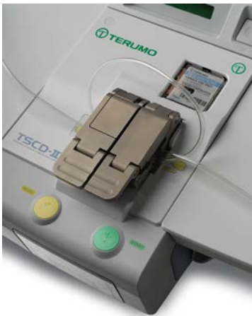
Figure 5-5: Sample coil loaded into the sterile tubing welder
