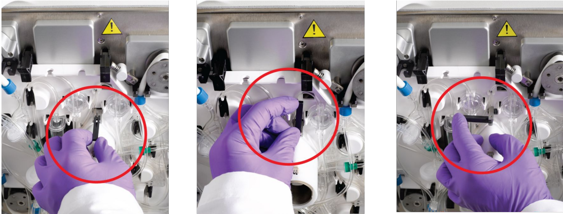
Figure 7-4: Securing the tubing organizer with an internal mounting clip
