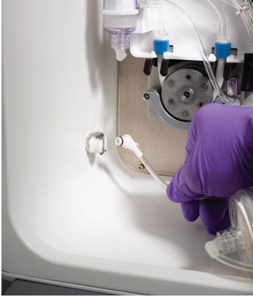
Figure 7-12: Connecting the gas inlet line
