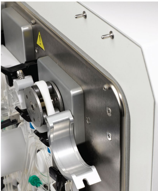
Figure 7-7: Tubing centered on the pump rotor
