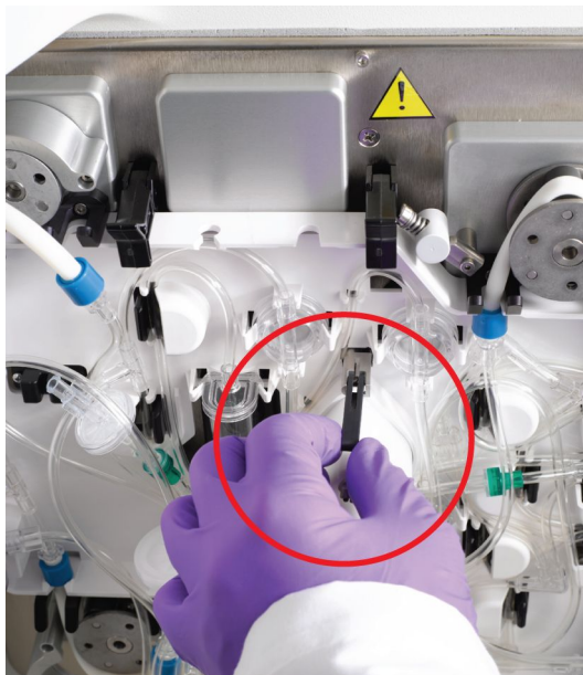
Figure 7-2: An internal mounting clip in the correct horizontal position
