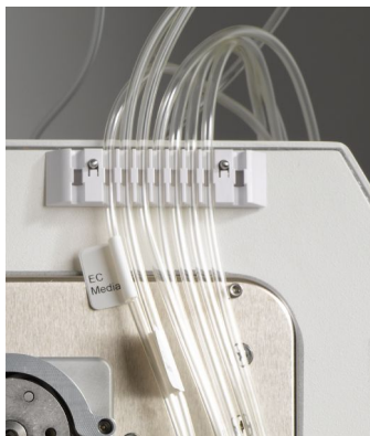
Figure 7-11: Tubing line guide properly attached
