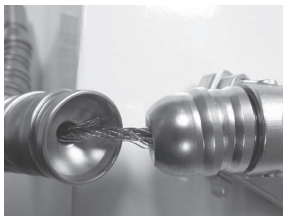
Figure 3 - Appearance of a fraying cable – DO NOT USE
