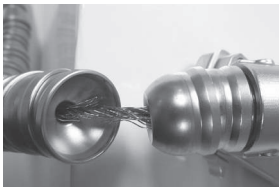
Figure 7 - Cable demonstrating fatigue and fraying
